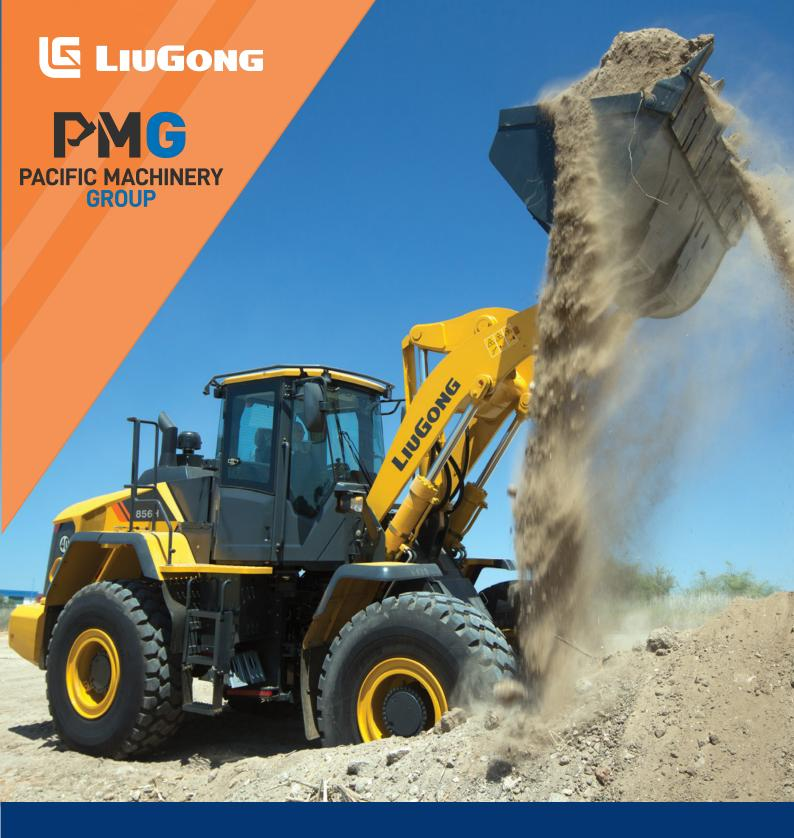
EngineCummins 6LTAA9.3Rated Power162 kW (220 hp / 217 ps) @ 2,200 rpmNet Power152 KW (204 HP / 207 PS) @ 2,200 RPMOperating Mass17,000 kgStandard Bucket Size3.0 M³Standard Breakout Force199 kNStandard Dump Clearance3,100 mm
